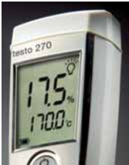
Figure 25: Visual and Audible alarm if a given limit is exceeded
