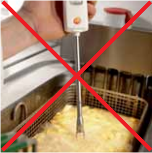
Figure 30: Correct measurement results only possible if measurement is taken without the product being deep fried!
